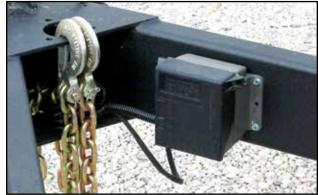
Fig 52 - Break-Away system control box
