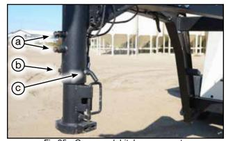
Fig 25 - Gooseneck hitch components
