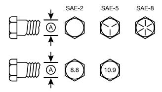
Torque figures indicated above are valid for non-greased or non-oiled threads and heads unless otherwise specified. Therefore, do not grease or oil bolts or capscrews unless otherwise specified in this manual. When using locking elements, increase torque values by 5%.
