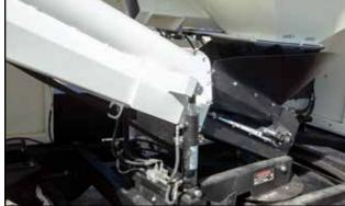
Fig 36 - Move the tube into position
