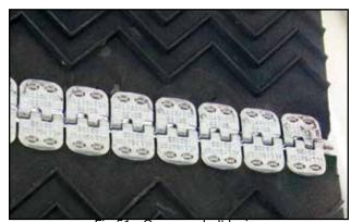
Fig 51 - Conveyor belt lacing
