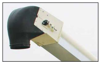
Fig 42 - Discharge roller bearing
