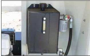
Fig 46 - Hydraulic oil reservoir and filter
