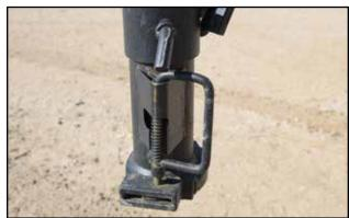
Fig 26 - Gooseneck trailer coupler
