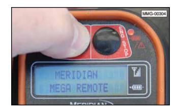
If the "NO LINK" message appears, the remote control handset is not communicating with the control panel on the seed tender. Make sure the ON/OFF key switch is in the ON position.
