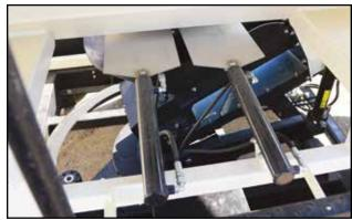
Fig 30 - Compartment slide gates
