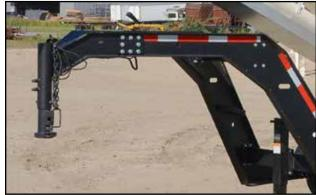
Fig 23 - Gooseneck hitch
