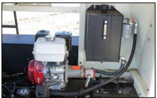
Fig 44 - Engine and hydraulic reservoir
