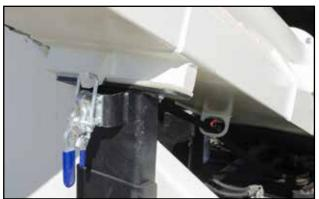
Fig 20 - Conveyor tube transport lock
