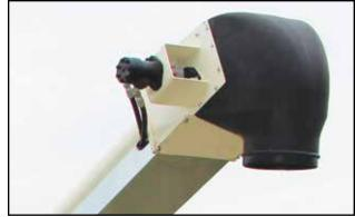
Fig 11 - Conveyor delivery spout
