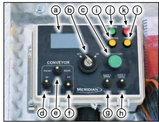
Fig 17 - Electrical control panel inside box
