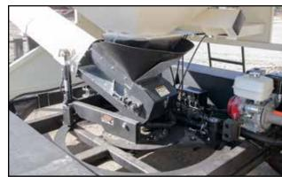
Fig 8 - Conveyor tube turret
