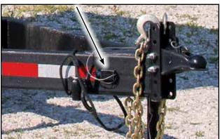
Fig 16 - Break-Away cable on hitch tongue
