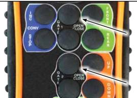
Fig 38 - Open/close gates from remote control
