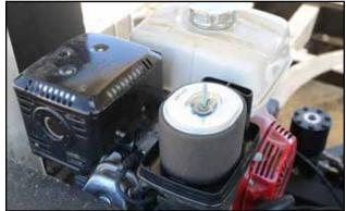
Fig 41 - Engine air filter
