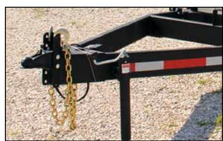
Fig 14 - Tongue on a bumper hitch trailer
