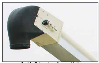
Fig 49 - Drive roller adjustment bolt
