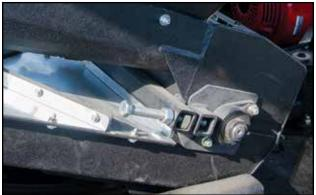
Fig 48 - Idler roller tension bolt at the bottom of belt
