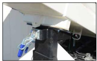
Fig 35 - Unlock the conveyor tube
