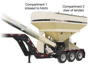
Fig 19 - Compartment position identification
