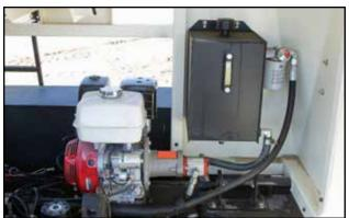
Fig 7 - Engine, hydraulic oil reservoir and filter
