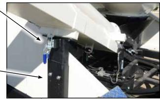
Fig 9 - Conveyor tube transport cradle and lock
